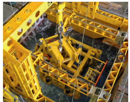
4. ábra. Module Handling System in Moonpool
